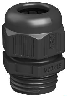
The quickest and most convenient way of providing strain relief and tightness with cable glands on junction boxes and housings is with the tried-and-trusted V-TEC VM cable glands from OBO. A protection rating of IP68 is achieved through the integrated sealing lip and the special OBO slat  $\,$ technology. Strain relief and tightness have been tested to DIN EN 62444.
