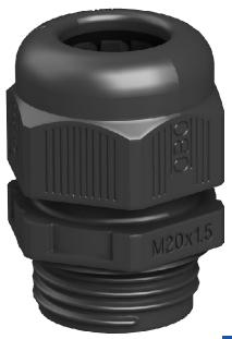
The quickest and most convenient way of providing strain relief and tightness with cable glands on junction boxes and housings is with the tried-and-trusted V-TEC VM cable glands from OBO. A protection rating of IP68 is achieved through the integrated sealing lip and the special OBO slat  $\,$ technology. Strain relief and tightness have been tested to DIN EN 62444.
