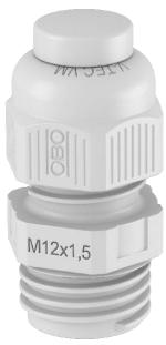
The quickest and most convenient way of providing strain relief and tightness with cable glands on junction boxes and housings is with the tried-and-trusted V-TEC VM cable glands from OBO. A protection rating of IP68 is achieved through the integrated sealing lip and the special OBO slat  $\,$ technology. Strain relief and tightness have been tested to DIN EN 62444.
