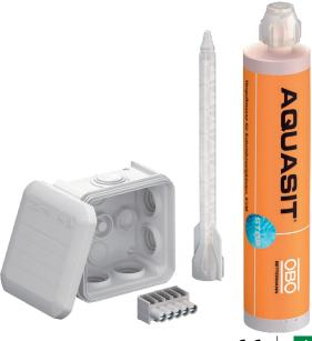
Junction box set with terminal strip for the connection of cables and lines indoors and in protected outdoor areas. Including Aquasit cold casting compound, IP68 protection rating Square design with plug-in seals to the sides and knock-out entries in the bottom. Suitable for wall and ceiling mounting and on mounting panels. With the option to fasten inside. With fixed clamping cover. Made from halogen-free materials.
