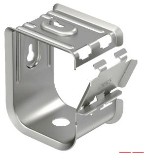
Metal cable tidy for high mechanical stability, even in case of fire. Suitable for safe mounting above fire protection ceilings. Also approved as a cable-specific variant for the maintenance of electrical functionality to DIN 4102 part 12. For wall and ceiling mounting. The lock can be opened
