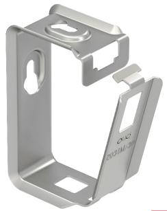
Metal cable tidy for high mechanical stability, even in case of fire. Suitable for safe mounting above fire protection ceilings. Also approved as a cable-specific variant for the maintenance of electrical function to DIN 4102 part 12. For wall and ceiling mounting. Lock can be opened without tools. Detailed information on the approved routing variants can be found in the appropriate testing
