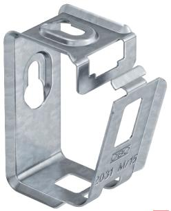
Metal cable tidy for high mechanical stability, even in case of fire. Suitable for safe mounting above fire protection ceilings. Also approved as a cable-specific variant for the maintenance of electrical function to DIN 4102 part 12. For wall and ceiling mounting. Lock can be opened without tools. Detailed information on the approved routing variants can be found in the appropriate testing documentation.
