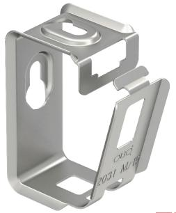
Metal cable tidy for high mechanical stability, even in case of fire. Suitable for secure mounting above fire protection ceilings. Also approved as a cable-specific variant for the maintenance of electrical function to DIN 4102 part 12. For wall and ceiling mounting. Lock can be opened without tools. Detailed information on the approved routing variants can be found in the appropriate testing documentation.
