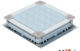
Underfloor junction and branch box for screed-covered underfloor installation ducts with sheet steel side walls. To mount installation units in the mounting lid (to be ordered separately). Height can be infinitely adjusted to the nominal screed height (rapid adjustment possible) and the screed can be worked flush to the screed scraping edge. With noise decoupling option after screed laying and can be used with system accessories, also for heavy-duty application.
