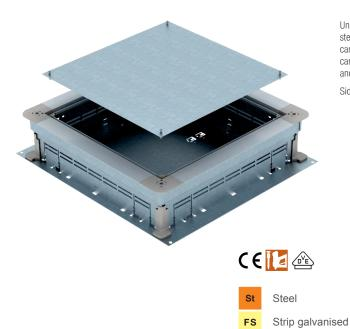
Underfloor junction and branch box for screed-covered underfloor installation ducts with sheet steel side walls. To mount installation units in the mounting lid (to be ordered separately). Height can be infinitely adjusted to the nominal screed height (rapid adjustment possible) and the screed can be worked flush to the screed scraping edge. With noise decoupling option after screed laying and can be used with system accessories, also for heavy-duty application.
