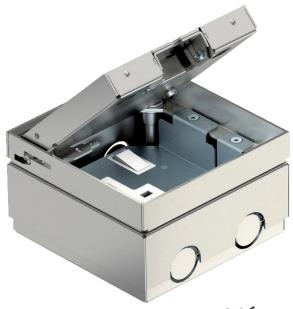
Square installation unit for use in dry-care cavity and screed floors in indoor areas. With recess in the hinged lid for the floor covering. Installation housing with pre-marked insertion openings for pipes (M25). Cover adjustable to top edge of floor covering using four height-adjustment supports. The minimum installation depth is 85 mm, the height adjustment range +20 mm.
