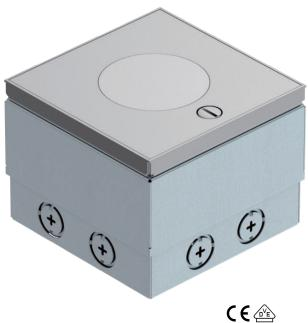
Square floor socket for use in wet-care cavity and screed floors in indoor areas. Cable exit for height-adjustable tube body. Installation housing with pre-marked insertion openings for pipes (M20/M25). Cover adjustable to top edge of floor covering using four height-adjustment supports. The minimum installation depth is 110 mm, the height-adjustment range is +25 mm. The load-bearing capacity of 15 kN is only guaranteed when in an unused state.
