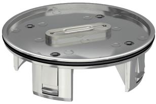
Height-adjustable cord outlet for installation in RKF frame cassettes and in height-adjustable round and square RKFR and RKFN cassettes. Raised height when used, flushfloor when unused. Use in wet-care floors. With 4 mm floor covering recess for construction-side panelling with cut resistant floor covering, with handle clamp.
