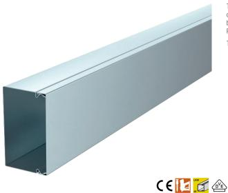
Trunking cover and base with base perforation. Equipotential bonding is guaranteed between the cover and the base without any additional aids. The LKM cable trunking, type LKM 60100FS, has been tested for the maintenance of electrical functions as a routing system according to DIN 4102 Part 12. Please note the cable types tested in the BSS fire protection systems division!
