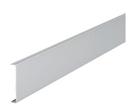
Aluminium cover, for closing Rapid GA device installation duct and ISS service poles with a 76.5 mm system opening. The firm position of the cover and electrical contact to the lower part of the duct and service pole is guaranteed thanks to type RKV3V locking brackets. There are 6 premounted locking brackets included per delivery length (2,000 mm).
