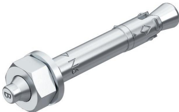
The nail anchor N can be used for multiple fastenings of non-load-bearing systems and in cracked and non-cracked concrete, thereby combining the benefits of a bolt tie with even easier mounting. The nail tie only needs to be hammered into the drill hole. It is not necessary to apply torque subsequently. When the load occurs, the nail tie spreads itself and bolts itself in the drill hole.
