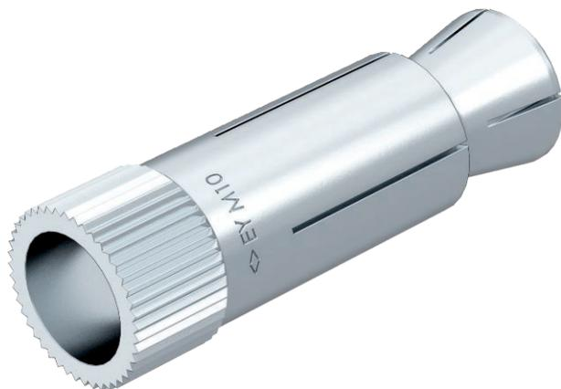
Hollow core anchor "Easy" for mounting in prestressed hollow concrete slabs. When the screw or the nut is tightened, the cone is released from the anchor sleeve and pulled into it. This makes the anchor expand in the hollow space, thereby creating firm lock. The hollow core anchor can also be used when the expansion area is not located in the cavity.
