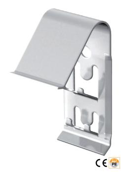
Cover clamp for universal fastening of covers on cable trays, mesh cable trays and AZ small ducts. Depending on the tray width, 4-6 cover clamps are required for secure fastening of a 3 m cover. The cover clamp is not suitable for use with mesh cable trays with a side height of 35 mm.
