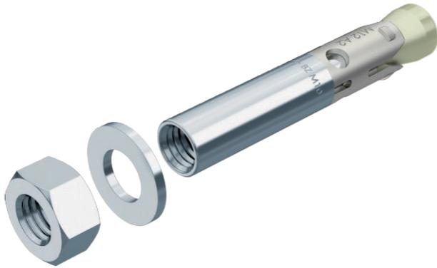
Bolt tie BZ-IG with internal thread for the anchoring of medium-duty to heavy-duty loads, both in cracked and non-cracked concrete. It combines high approved loads with small edge distances and axial spacings. Undercutting the drill holes is not necessary.
