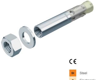
Bolt tie BZ-IG with internal thread for the anchoring of medium-duty to heavy-duty loads, both in cracked and non-cracked concrete. It combines high approved loads with small edge distances and axial spacings. Undercutting the drill holes is not necessary.
