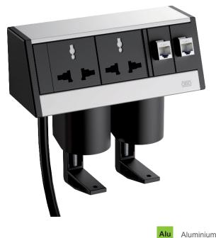
The DB Deskbox ensures a direct supply of the workplace with power, data and multimedia technology and is suitable for fixed attachment to a tabletop. The Deskbox is equipped with a connection cable, which runs out of the profile from below. The housing consists of an anodised, silver-coloured aluminium profile.
