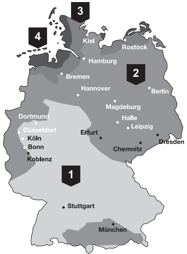
Wind zones in Germany as per DIN EN 1991-1-4 NA (country-specific)
