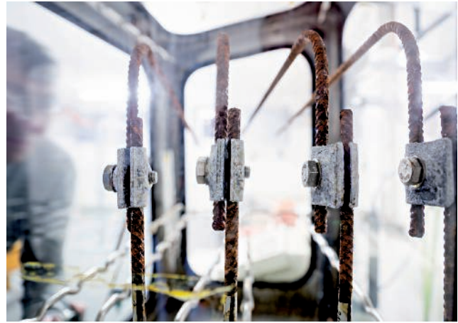
BET SO 2 testing system
