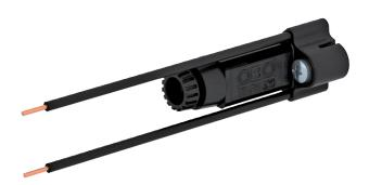
Fuse holder with bayonet lock for fine-wire fuse for dimensions  $\emptyset$  5 x 20 mm. Connection wires that maintain electrical functionality with nominal cross-section 2.5  $\,\text{mm}^2$  , ready-stripped. For mounting on one of the exposed domes in the junction box of the FireBox T series using the  $\,$ supplied screw.
