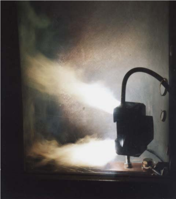
Fig. 4 Class I arrester with open metal electrodes and under test with a current of 400A/0,5s.
