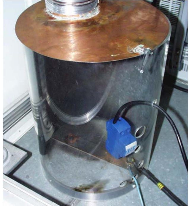
Fig. 6 Class I N-PE spark gap with graphite electrodes in a sealed housing under test with a current of 400 A/0,5s.
