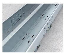
Mounting of separating retainer The barrier strip type TSG is screwed by means of coach bolts in the bottom of the cable tray. Depending on the width of the cable tray system multiple partitions can be used. Here, the divider serves as a lid support.
