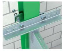
Clamp fixing of heavyweight bracket Clamp fastening of a heavy-duty bracket with clamping angles or clamping lugs on a vertical steel girder.
