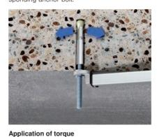
Fastening of the threaded rod by tightening the hexagon nut with the specified torque in the approval.
