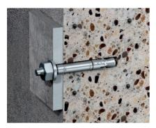
Nail anchor, type N, with threaded connection Nail anchor, type N, with M6 threaded connection, usable in cracked or non-cracked standard concrete C20/25 to C50/60.
