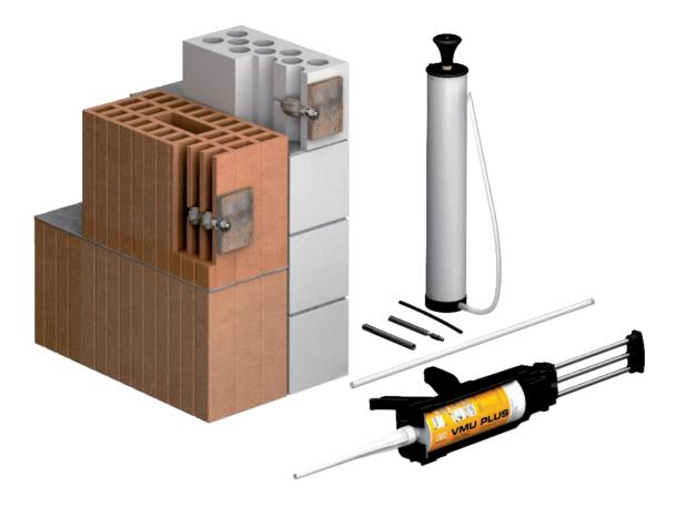
The VMS Plus injection mortar system is particularly suitable for fire-protection fastening in hollow brick, concrete, calcareous limestone, sand-lime brick and masonry. The non-spreading connection is created through the use of the plastic wire sleeve and a threaded anchor rod. The components are tested and approved for a fire-resistance period of 90 minutes.
