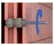
**Inserting the anchor rod** Attach the anchor rod in the filled wire sleeve up to the set marking. The mortar pushes through the openings of the wire sleeve, forming a closure.
