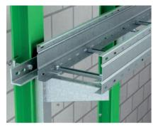
Wall bracket, heavy-duty Installation of the heavy-duty wall bracket, type AWSS, with clamping angle, type KWS, to steel girder to accept a wide span system. The wall bracket can also be mounted on concrete walls with anchor bolts.
