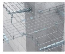
**Creation of a mesh cable tray cross-over** After cutting the side rails and bending the straps, the corner connector, type GEV 36, and the joint connector, type GSV 34, can be used to create cross-overs.
