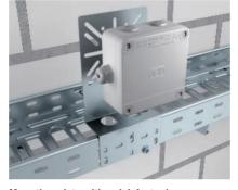
Mounting plate with quick fastening Fastening of the mounting plate, type MP, on the cable tray. The mounting plate can be fastened to the rail with quick connectors, and permanently fastened using truss-head bolts of type FRS B.
