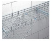
**Creation of a vertical exit** After cutting the mesh cable tray base, the vertically branching, cut mesh cable tray can be fixed using the joint connector, type GSV 34.
