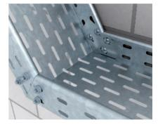
**Creating a height increase or decrease** After cutting into the side rail, the cable tray is bent manually at an angle of 0-60° and fixed with the straight connector RLVKV 60 FS. It is not necessary to cut into the bottom plate.
