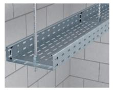
Centre suspension application Centre suspension of the cable tray systems MKS, SKS, EKS, DKS and IKS with a central suspension hanger, type MAH, and threaded rod 2078/M10.
