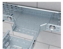
**Mounting of Magic T branch piece** Mounting of fittings by simple interconnection. For this, the cable tray with the spring side is locked into the fitting connection from above.
