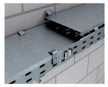
Screwless cover fastening with cover clamp Screwless cover mounting takes place with covers and the cover clamps, type DKU. The cover clamp is simply fixed in the perforation of the cable tray.
