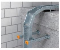
**Installation of falling adjustable vertical bend** Adjustable vertical bend to bridge height offsets. The adjustable vertical bend is connected with to the cable tray using the adjustable connectors.
