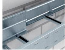
Screwed barrier strip fastening Barrier strip mounting in wide span cable ladders. Fasten using slide nuts and hexagonal bolts.
