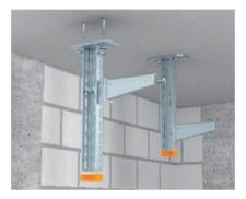
Standard mounting of suspended support with wall bracket, single-sided without spacer Cover fixing of a suspended support with single-sided bracket fixing. No spacer is required for widths up to and including 300 mm.
