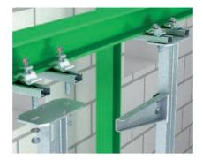
Steel clamping with C profile, route in transverse direction I support with welded head plate mounting, clamped to steel girder with C profile and TKH-L-25 chuck jaw. Tray route transverse to steel
