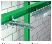
**Cable tray mounting on steel girder** Cable tray mounting with chuck jaws of type TKS-L-25 and U supports as cantilever beams on steel girders. Use spacers, type DSK, for safe functioning.
