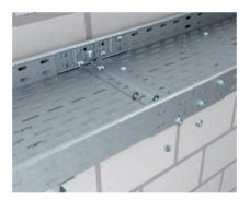
Straight connection with joint cover Cable tray with screwed straight connection and joint plate, type SSLB. The joint plate can also be mounted above the bar of the RV straight connector set.
