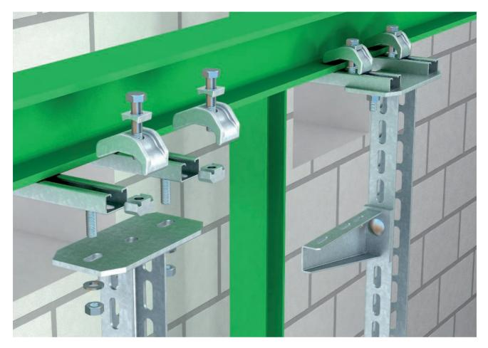
The clamp fastening systems with reduced installation times and work are a clear argument for the use of this system in all areas of professional electrical installations. Clamp fastening can be attached without difficult, of ten unpermitted drilling. The load range runs from light-duty clamping angles to heavy-duty chuck jaws.
