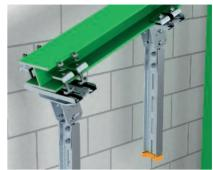
Head plate, variable (transverse) Installation of the variable, transversely adjustable head plate, type KI 8 VLP, on rising or falling steel structures with profile rail, type CPS 5 G and clamping angles, type KWH.
