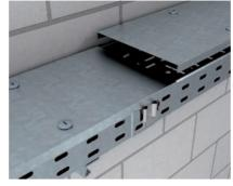
**Installation of cover with turn-buckle.** Cover with turn-buckles are fastened by turning the turn-buckle through 90°. Clamp fastening takes place under the rolled side rail of the cable tray.
