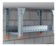
**Mounting example** Double-sided support mounting of U profiles with transverse traverse. Fastening of a wide span cable tray, type WKSG 110, with trusshead bolts on the transverse profile.
