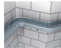
**Installation of bend (width 100 – 300 mm)** The bend in widths 100 to 300 mm is pushed into the rail on the one side and over the connector on the other. Additional supports should be planned for the area of the fittings.
