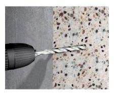
**Drilling** Making a hole of suitable diameter
