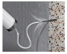
**Blowing out of the drill hole** Removing dust from the drill hole by blowing it out several times.
