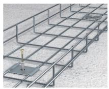
Direct floor fastening Direct floor mounting of mesh cable trays using clamp, type GKS 50.
