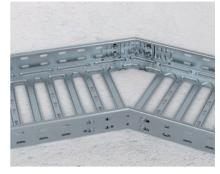
Creating a change of direction by cutting the cable tray Combine the cut trays and fix them from inside with two angle connectors, type RWVL.
