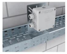
**Mounting plate with quick fastening** Fastening of the mounting plate, type MP, on the side rail of the cable tray. The mounting plate can be fastened to the rail with quick connectors, and permanently fastened using trusshead bolts of type FRSB 6x12 mm.
