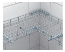
Creation of a mesh cable tray bend – angular After appropriate cutting of the mesh cable trays, they can, together with joint connectors, type GSV 34, and a bent slotted steel strap, be combined to a non-overlapping, angular mesh cable tray bend.
