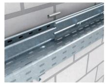
**Barrier strip mounting with screw connection** Screwed barrier strip fastening of the barrier strip, TSG 60, with truss-head bolts M6x12. The barrier strip can simply be run over the joint and connected without bolts using the barrier strip connector TSGV.
