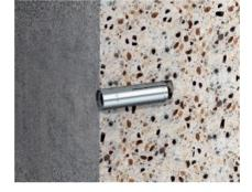
Drop-in anchor, type E Drop-in anchor, type E, with M8, M10, M12 internal thread. To accept small loads, approved for multiple fixings in cracked and non-cracked concrete of non-load-bearing systems.
