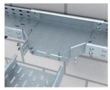
**Installation of tee (width 100 – 300 mm)** The tee in widths 100 to 300 mm is pushed into the rail on the one side and over the connector on the other. Additional supports should be planned for the area of the fittings.
