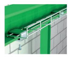
Installation of mesh angle Fastening of the mesh angle, type GW 40/80, to steel girders using beam clamps, type KL 20 or KL 30.
