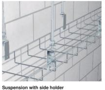
Suspension with side holder Suspension of a mesh cable tray with side holders, type SH M 10 and threaded rods, type 2078/M10.
