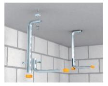
Installation of TP support with single-sided bracket fixing
