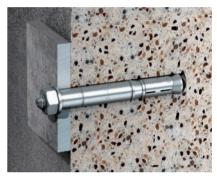
Heavy-duty anchor, type SZ Heavy-duty anchor, type SZ, with M12 thread connection for fastening components with high loads, approved for cracked and non-cracked standard concrete C20/25 to C50/60.
