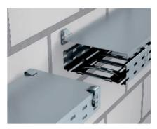
Screwless cover mounting Screwless installation of the cover, type DRLU, on a cable tray using the cover clamp, type DKU. The cover clamp locks in the top hole of the side rail.
