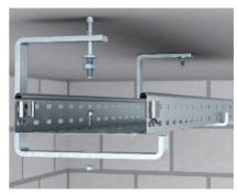
**Direct fastening of the ceiling bracket** Direct mounting of the AHB ceiling bracket with anchor bolt on the ceiling. Maximum cable tray width 400 mm.
