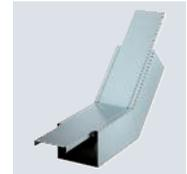
45° vertical bend, rising version, with intumescent fire protection mesh for PYROLINE® Rapid PLM installation duct. Suitable for direct wall and ceiling mounting, mounting below system floors and on support systems. Tool-free joint mounting with PLM SI joint connector. The cover is snapped on without tools, allowing rapid inspection and retroassignment. The cover overhang allows offset cover mounting for continuous equipotential bonding of the entire duct section.
