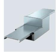
Reducer with intumescent fire protection mesh for symmetrical reduction of straight duct sections from PLM D 0810 to PLM D 0410. Suitable for direct wall and ceiling mounting, mounting below system floors and on support systems. Tool-free joint mounting with PLM SI joint connector. The cover is snapped on without tools, allowing rapid inspection and retroassignment. The cover overhang allows offset cover mounting for continuous equipotential bonding of the entire duct section.
