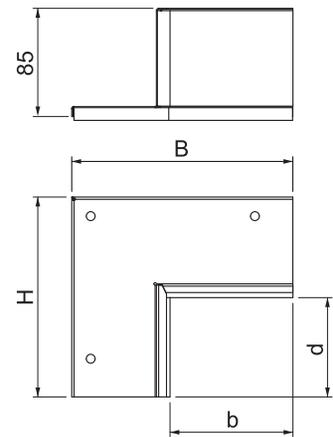
Wall connection collar, 4-sided, duct height 80 mm
