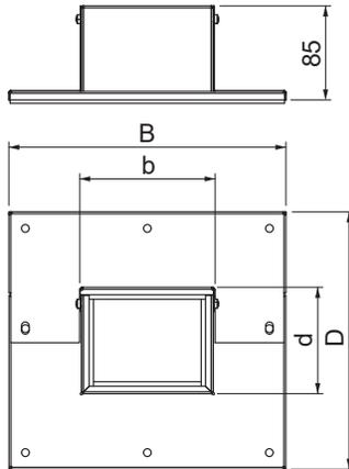
End piece, duct height 80 mm
