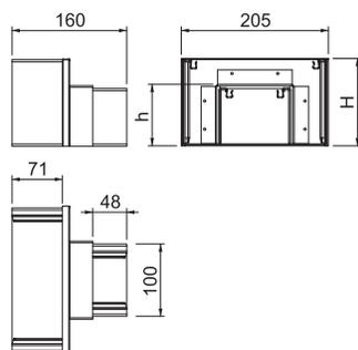
Wall connection set, double-sided, for corner mounting, duct height 120 mm
