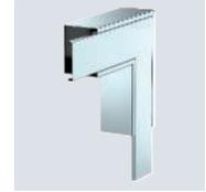
Flat angle with intumescent fire protection mesh for PYROLINE® Rapid PLM installation duct. Suitable for direct wall and ceiling mounting, mounting below system floors and on support systems. Tool-free joint mounting with PLM SI joint connector. The cover is snapped on without tools, allowing rapid inspection and retroassignment. The cover overhang allows offset cover mounting for continuous equipotential bonding of the entire duct section.
