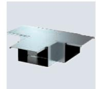
T branch piece with intumescent fire protection mesh for PYROLINE® Rapid PLM installation duct. Suitable for direct wall and ceiling mounting, mounting below system floors and on support systems. Tool-free joint mounting with PLM SI joint connector. The cover is snapped on without tools, allowing rapid inspection and retroassignment. The cover overhang allows offset cover mounting for continuous equipotential bonding of the entire duct section.
