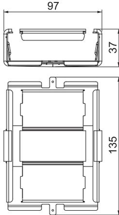
Joint connector set, duct height 80 mm
