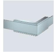
External corner with intumescent fire protection mesh for PYROLINE® Rapid PLM installation duct. Suitable for direct wall and ceiling mounting, mounting below system floors and on support systems. Tool-free joint mounting with PLM SI joint connector. The cover is snapped on without tools, allowing rapid inspection and retroassignment. The cover overhang allows offset cover mounting for continuous equipotential bonding of the entire duct section.
