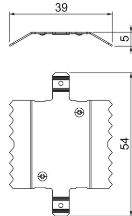
Joint connector set, duct height 40 mm
