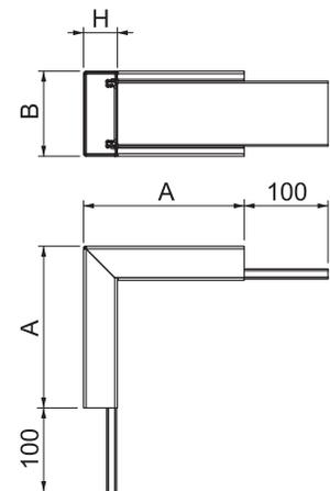
Flat angle, duct height 40 mm
