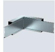
Internal corner with intumescent fire protection mesh for PYROLINE® Rapid PLM installation duct. Suitable for direct wall and ceiling mounting, mounting below system floors and on support systems. Tool-free joint mounting with PLM SI joint connector. The cover is snapped on without tools, allowing rapid inspection and retroassignment. The cover overhang allows offset cover mounting for continuous equipotential bonding of the entire duct section.
