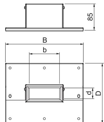
End piece, duct height 40 mm
