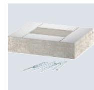
End piece for PYROLINE® Con D EI90 fire protection duct, consisting of fibre glass light concrete which is resistant to water and frost for closing the duct ends.
