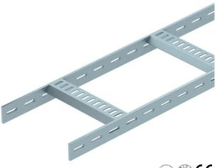
Shipbuilding cable ladder with perforated side rail of side height 40 mm with welded, perforated trapezoidal rungs which open in a downwards direction. Load tested according to IEC in conjunction with connector, type SLV. The shipbuilding cable ladder, including fittings, is also available in stainless steel
