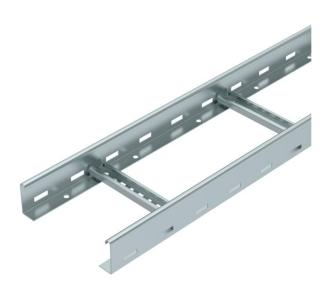
Cable ladder with 60 mm side height with welded C30 profile rungs which are open in an upwards direction. Rolled side rail for reinforcement and as edge protection. Fastening to the bracket takes place using clamps, type LKS 40. The slot dimension of the frame is 16.5 mm and the appropriate clamp clip is type BS-H...
