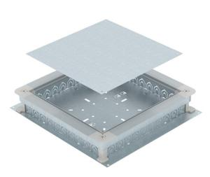
Underfloor junction and branch box for 10 installation pipes on each side (M20 or M32) with sheet steel side walls. To mount installation units in the mounting lid (to be ordered separately). Height can be infinitely adjusted to the nominal screed height (rapid adjustment possible) and the screed can be worked flush to the screed scraping edge. With noise decoupling option after screed laying and can be used with system accessories, also for heavy-duty application.
