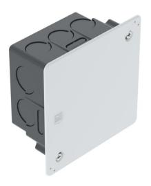
Flush-mounted connection box for clamping terminals, for use in masonry with an installation depth of at least 45 mm. With cover and cover screws (15 mm). Flat cover edge, roughened surface.
