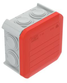
Junction box for the connection of cables indoors and in protected outdoor areas. Square design with plug-in seals to the sides and knock-out entries in the bottom. Suitable for wall and ceiling mounting and on mounting panels. With the option to fasten inside. With fixed clamping cover. Made from halogen-free, UV-resistant materials.
