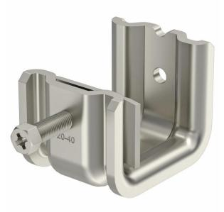
This type of support clamp is pushed onto the support and fixed to the girder or flat iron using a pressure trough and bolt (M8). The hexagonal bolt has a WAF of 10 mm. In the clip element also two more M8 threads are introduced, for example to attach threaded rods.
