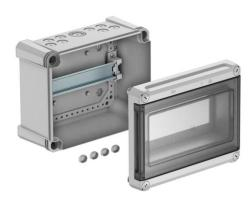
Distribution box for surface mounting, for the current sub-distribution in interior and protected exterior areas, in accordance with IEC 439-3. With pre-mounted 35 mm hat profile rail. IP66 protection type and IK07 protection rating. Transparent cover to screw on, with cut-out.
