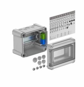
Distribution box with terminal strip for surface mounting, for the current sub-distribution in interior and protected exterior areas, in accordance with IEC 439-3. With pre-mounted 35 mm hat profile rail. IP66 protection type and IK07 protection rating. Transparent cover to screw on, with cut-out.
