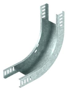
$90^\circ$  rising vertical bend, for all cable tray types of 35 mm side height. The vertical bend is pushed over the end of the cable tray and screwed tight. Fastening materials should be ordered separately.
