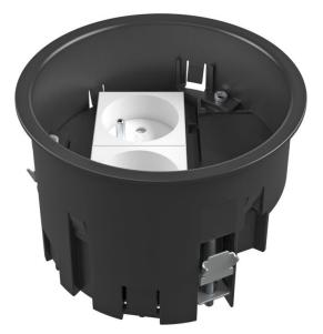
Installation socket for GES R2 floor socket for mounting in UD GES R2 screed box and in raised floor plates with an installation opening diameter of 122 mm.
