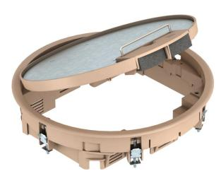
Service outlet with handle clamp for up to 10 individual Modul 45 devices in 2 UT3 and one UT4 universal support, use in duct systems and system floors for indoor use.
