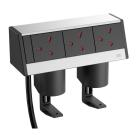
The DB Deskbox ensures a direct supply of the workplace with power, data and multimedia technology and is suitable for fixed attachment to a tabletop. The Deskbox is equipped with a connection cable, which runs out of the profile from below. The housing consists of an anodised, silver-coloured aluminium profile. The Deskboxes can be mounted simply on a tabletop with 2 fastening vices, without damaging the tabletop. Mounting is possible on a tabletop with a thickness of 8 to 40 mm.
