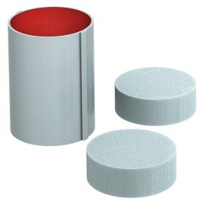
Internally coated pipe shells with click lock. The inner space can be fitted with cables and electrical installation pipes completely. For interior application. CE-labelled, European approved construction product according to ETA-13/0904 and German general type approval. Fire resistance up to 120 minutes.
