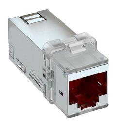
Connection module Cat. 6A (ISO) shielded, with an RJ45 slot. Including an EMC screen hood, a dust cover, a cable tie, a Keystone fastening frame and mounting instructions. Suitable for installation in the data technology supports of type DTG-2C and DTS-2C, support plate of type MTM 2C and MTM 3C, mounting plate of type MPR2 2C, mounting supports of type MTGE2 2C, MTGE2 15 2C and MT-GE2 F 2C.
