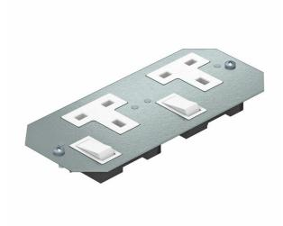
Cover plate with two switched single sockets for installation in mounting supports beneath GES service outlets and cassettes. Sockets with increased contact protection with screw connection, 3-pole, 13 A, 250 V $\sim$ , corresponds to BS 1363.
