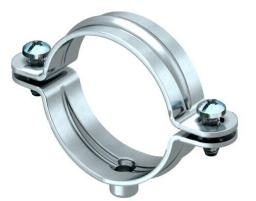
Mounting with screw-in spacer clips. Spacer clips and screw-in spacer clips are available in various materials: in V2A stainless steel, in electrogalvanised, hot-dip galvanised steel or in aluminium. Fastening can take place with bolt ties or angler anchors and Sprint screws.
