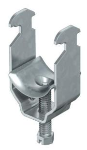
Suitable for all C profile rails with slot width 16–17 mm. Clip, bolt and pressure trough made of hot-dip galvanised steel. Version with welding and/or locknuts for use under difficult circumstances and for shake protection on request.
