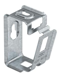
Metal grouped support for high mechanical stability, even in case of fire. Suitable for safe mounting above fire protection ceilings. Also approved as a cable-specific variant for the maintenance of electrical function to DIN 4102 Part 12. For wall and ceiling mounting. Lock can be opened without tools. Detailed information on the approved routing variants can be found in the appropriate testing documentation.
